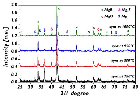
Figure 1. X-rays diffraction of MgB<sub>2</sub> powders, synthesized at different temperature, as reported in the graph
