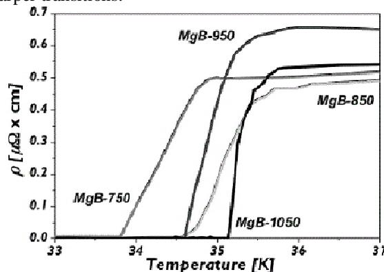
Figure 6.  $T_c$  of wire samples, ex-situ manufactured from the four powder samples. Samples synthesized at lower temperatures (MgB-750 and MgB- 850) show broader transitions due to the presence of unreacted Mg. Its content is reduced by synthesis temperature enhancement, and transition is sharper.
