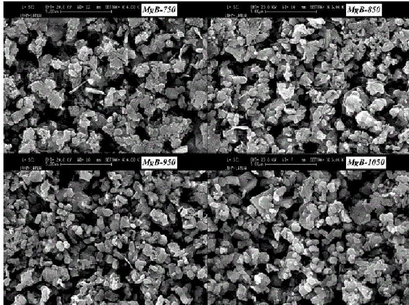
Figure 2. SEM Images of the four different samples. Images have been chosen as representative of the whole sample. In addition it has been reported the average grain size.
