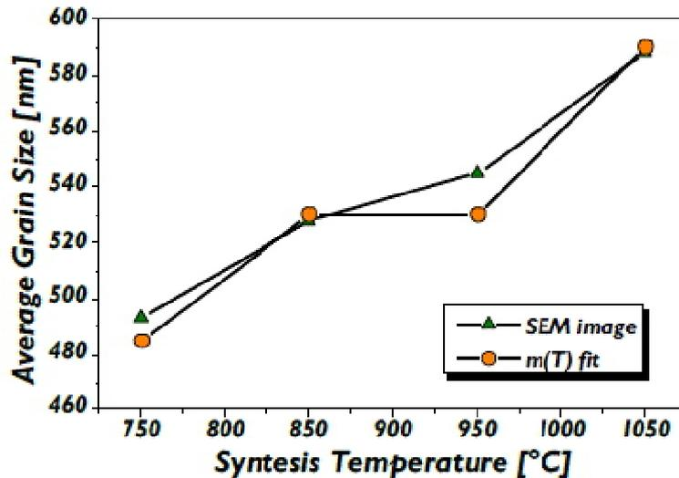
Figure 4. Average grain size measured from SEM images (green triangles) and fitting of magnetization curves (orange circles) in function of synthesis temperature
