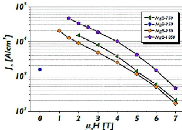
Figure 5.  $J_c$  of ex-situ manufactured wire samples using the four MgB<sub>2</sub> powders.
